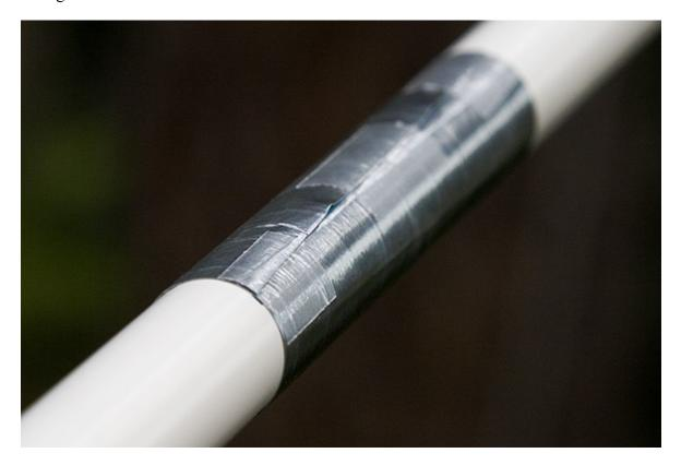
Before fixing the sleeve in place, check VSWR on 2m The sleeve should cause little if no change to 2m VSWR although it may appear to very slightly raise the resonant frequency; With the sleeve fitted, the VSWR should not be greater than 1.15:1 across the FM portion of band).
