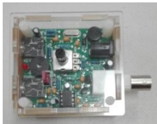
A Pixie 40M kitset CW transceiver was among some of the equipment that was on display at the CW workshop one Saturday morning.
