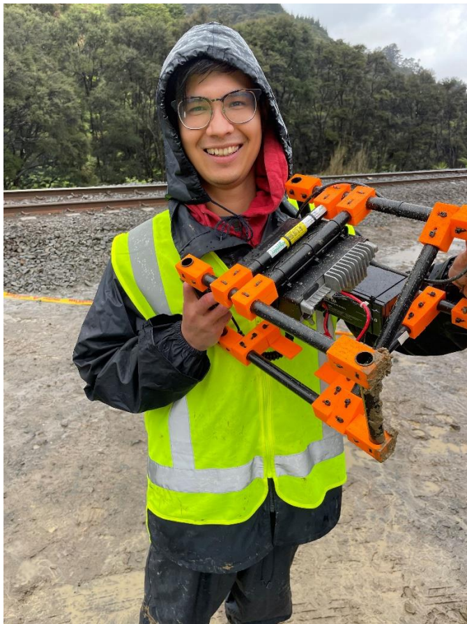
Above: Alec Lilley ZL1HAZ spend his Saturday under a gazebo sheltering from the heavy rain that was present for much of the day. He is seen here with the frame he built to hold his Tait mobile radio and battery for events such as this – he uses a 2m Flower Pot antenna he also built.
